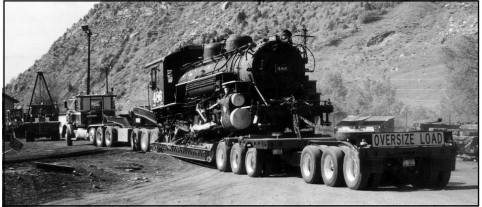
Engine 486 arrives in the D&SNG Durango yard on 5/22/99. The truck was placed over tracks, the trailer under the cab was detached and the trailer dropped to the rails. The locomotive was pulled off the ramp with another locomotive.
